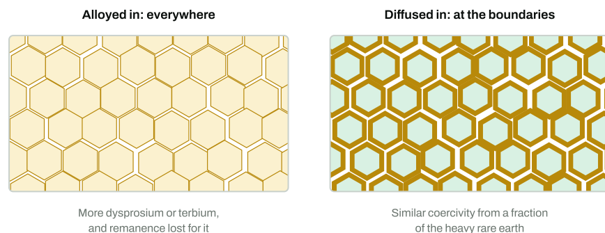
Figure 21. Grains of a sintered magnet, schematically. Amber is where the heavy rare earth sits; green is grain without it.
